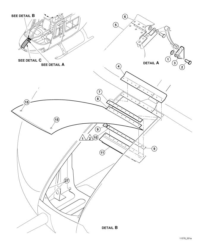
Figure 1 - Installation of Battery Door Assembly and Door Seal (Sheet 1 of 3)
