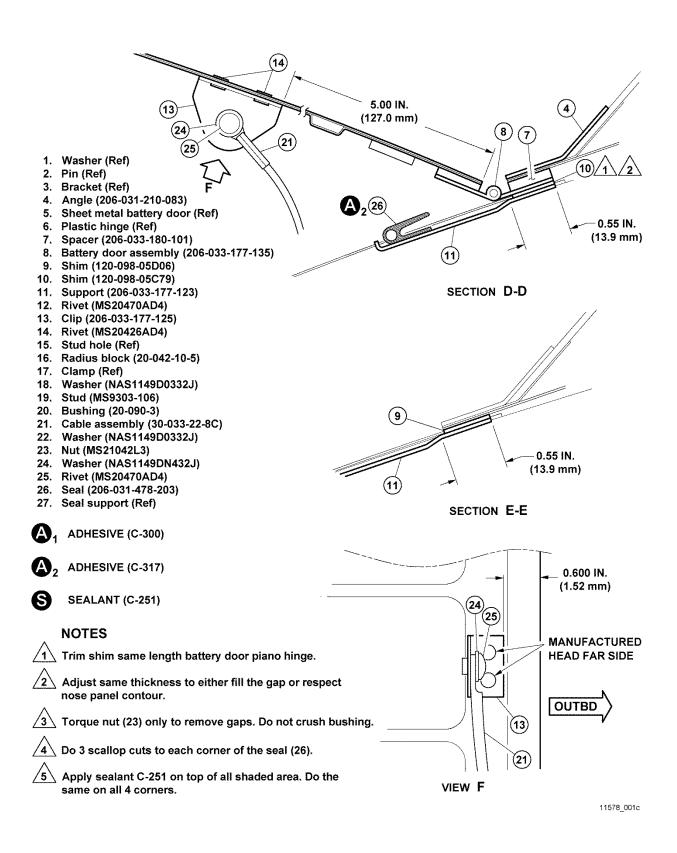
Figure 1 - Installation of Battery Door Assembly and Door Seal (Sheet 3 of 3)
