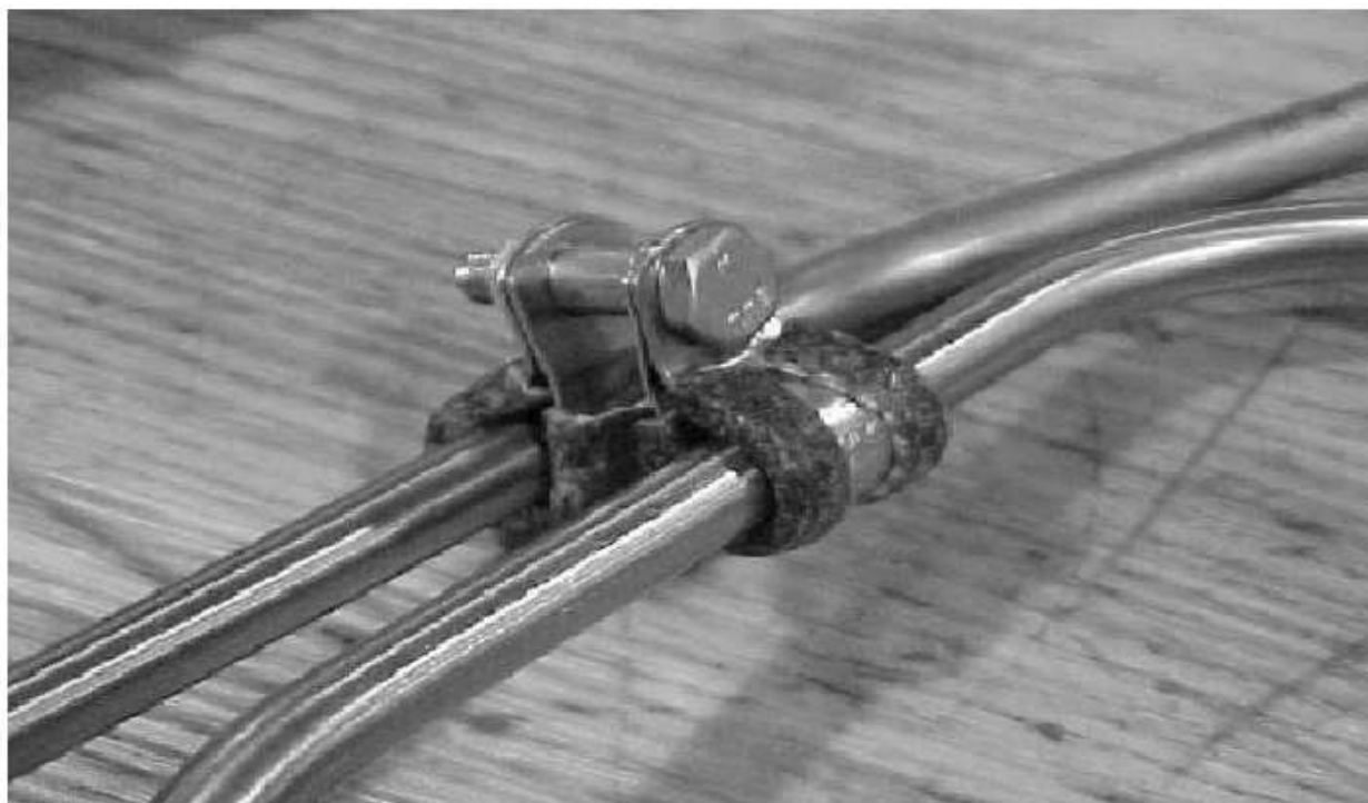
Properly Aligned Tube FIG. 6
