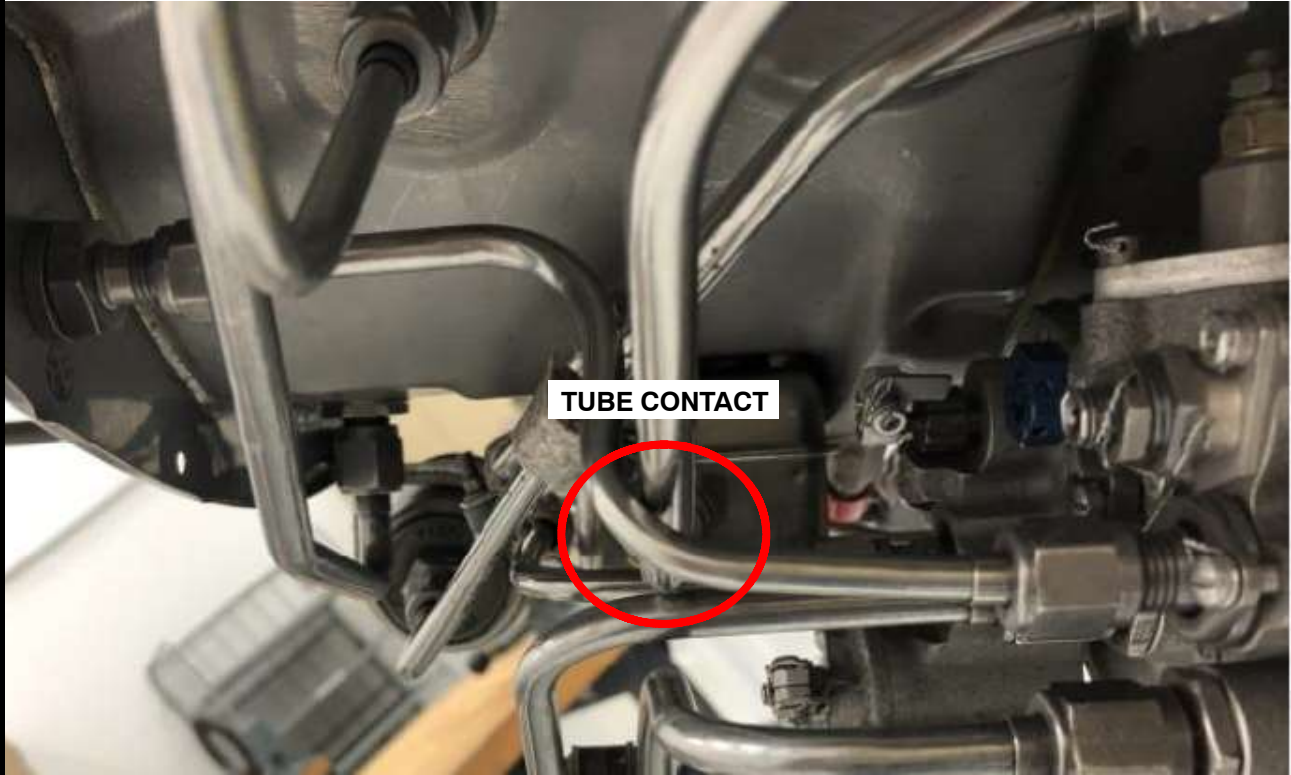
Incorrect Installation FIG. 13B
