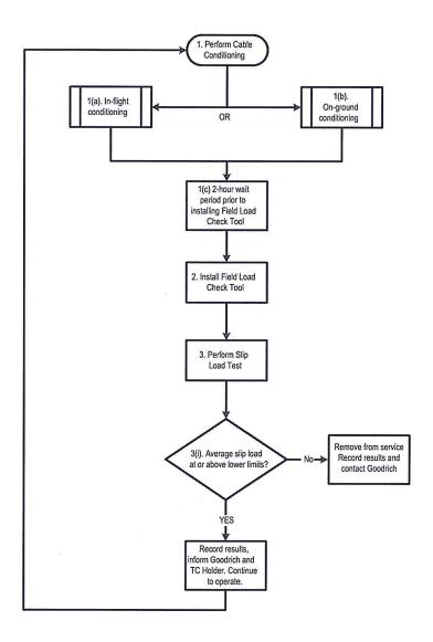
Figure 3. Load check flowchart
