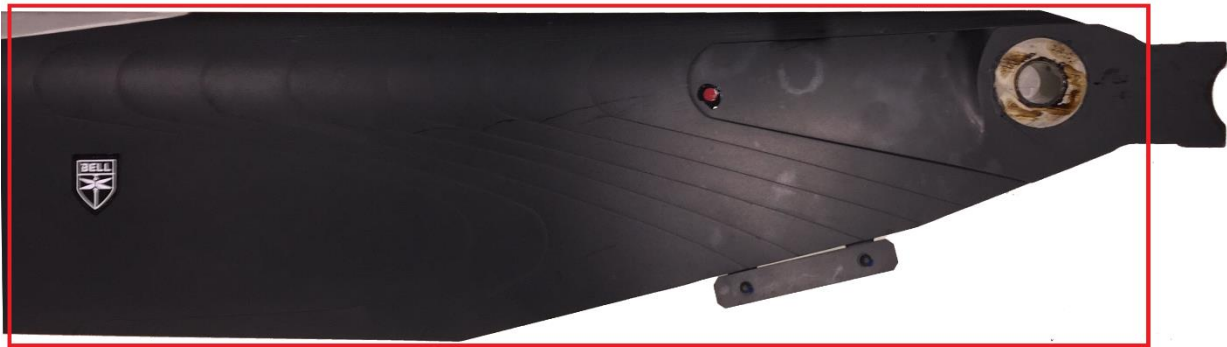
Figure 1. Area to be inspected with 3X- power magnifying glass, from STA 15.0 to STA 58.0 (upper and lower surfaces).
