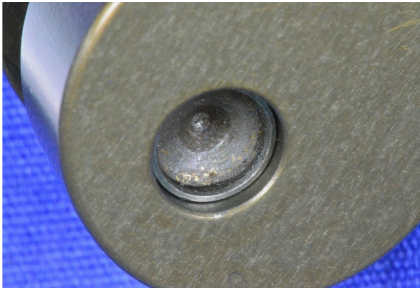
Figure 5 - Pivot Pin Out of Position
