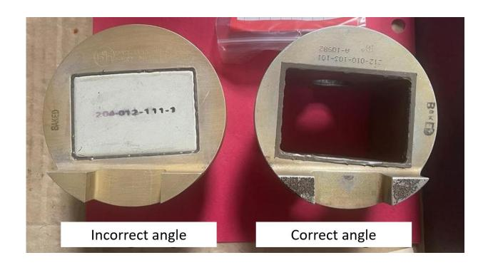
Figure 1. Inboard strap fitting 212-010-103-101.
