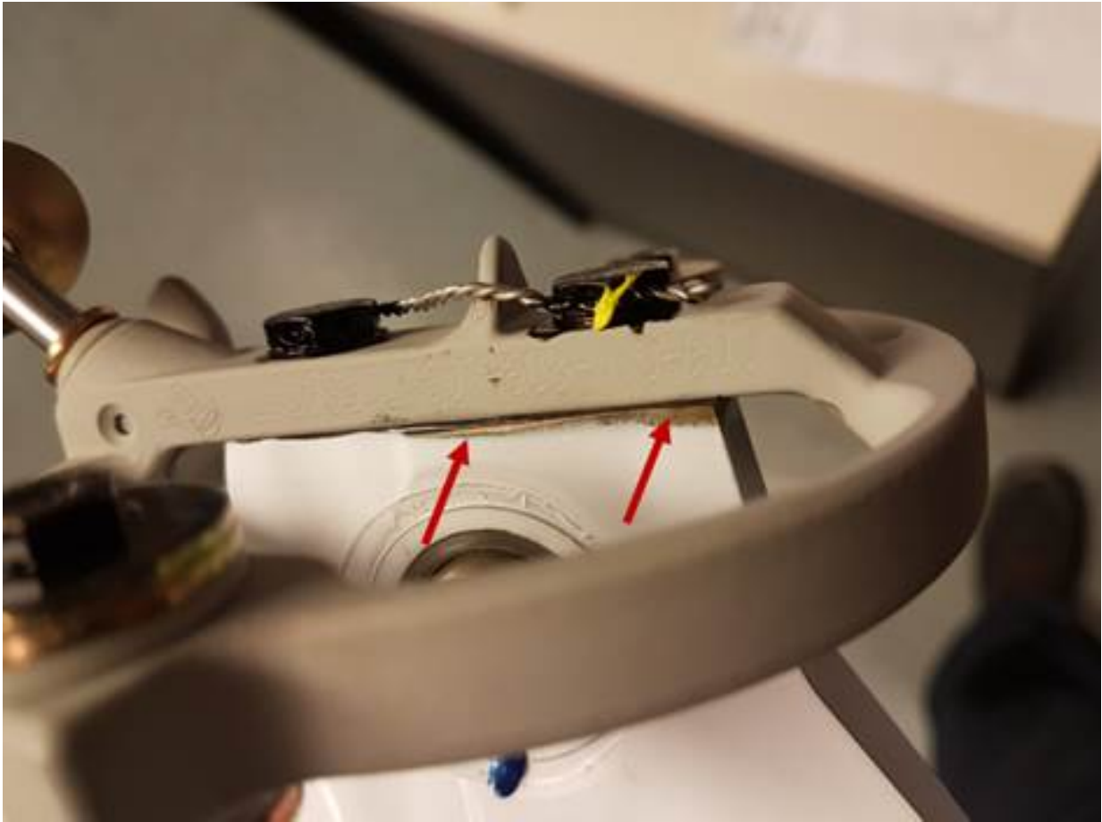
FIGURE 1 - Tail Rotor Blade Root End without Sealant
