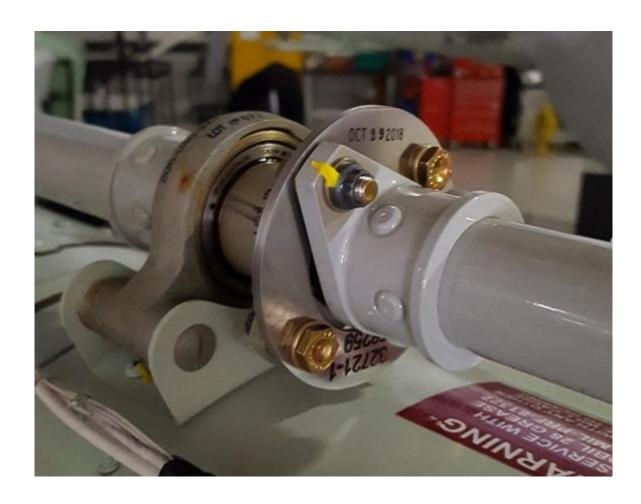
Figure 2 - Application of Torque Seal Lacquer (witness mark) (Shown as a yellow stripe from the nut to the adapter flange)
