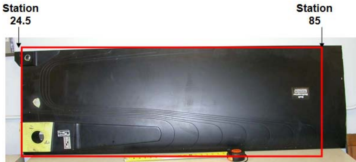
Figure 1 - Area to be inspected with 3X Power Magnifying Glass (Upper and Lower Surfaces)
