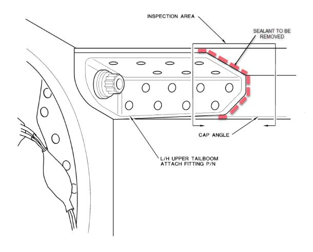
Figure 1. Fuselage Tailboom Attachment Inspection.
