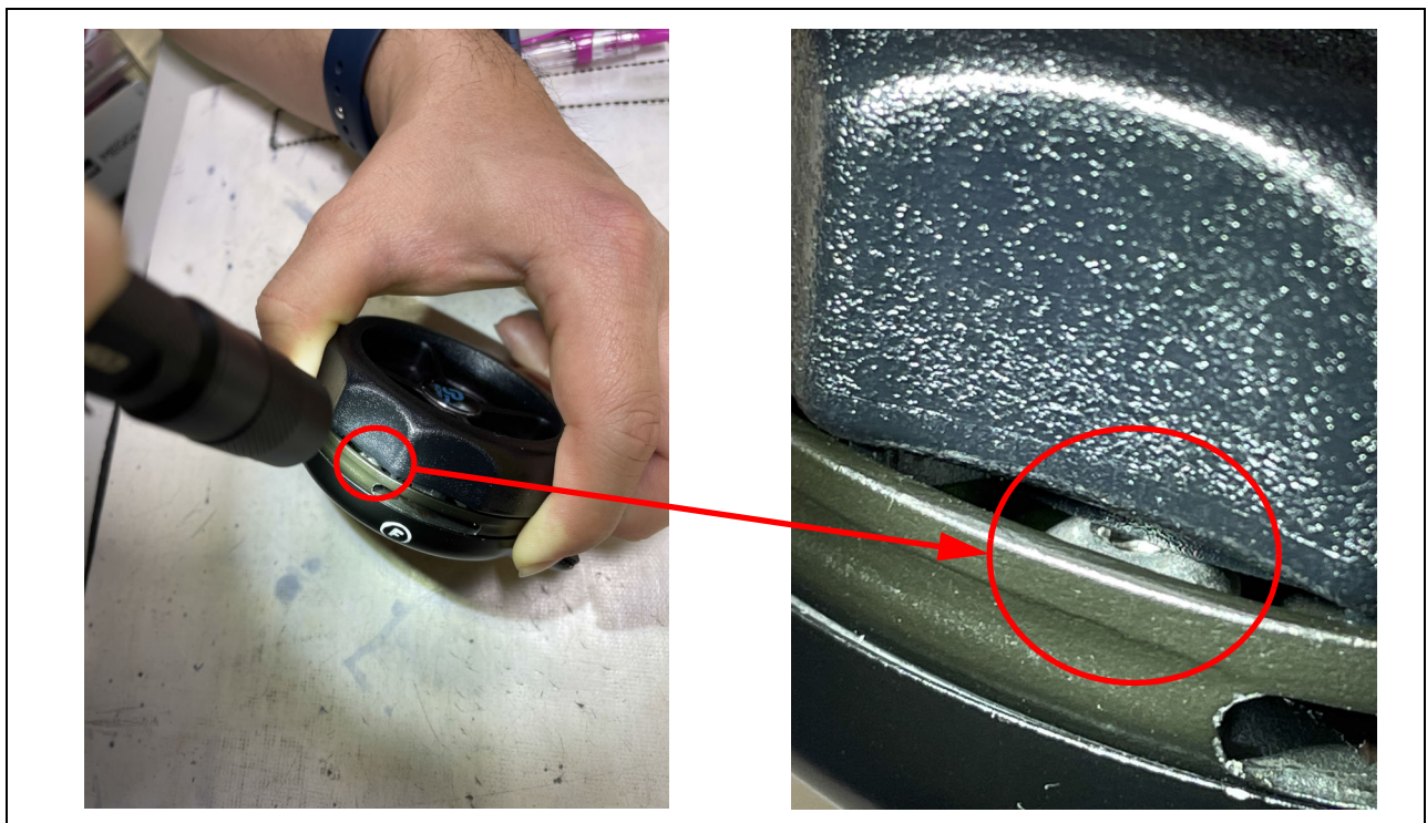
Figure 8 Side Belt Opening Inspection
