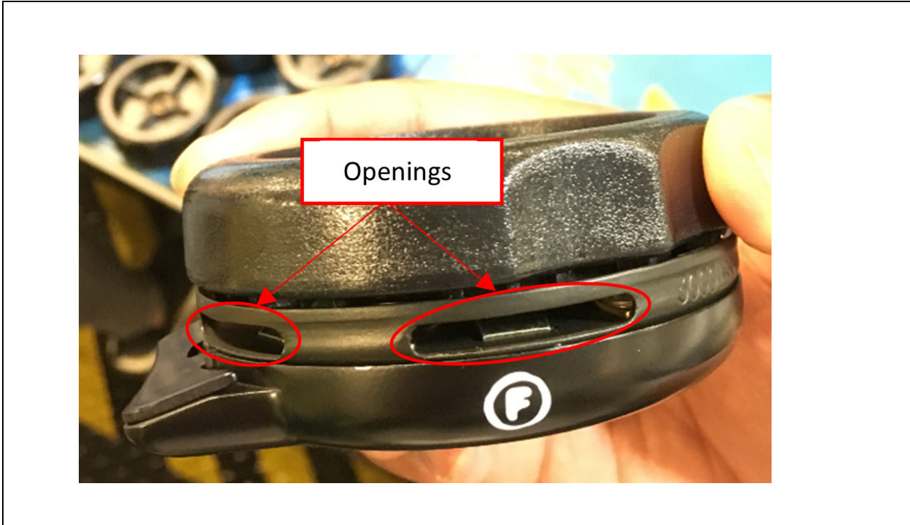
Figure 4 PNR 1111475 Series Rotary Buckle Openings for Inspection
