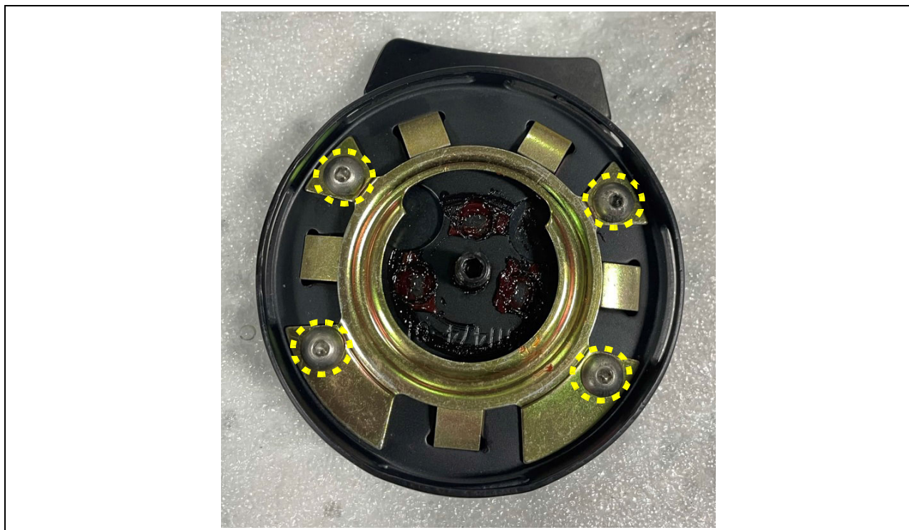
Figure 13 Disassembled Rotary Buckle with Suspect Torx Head Screws
