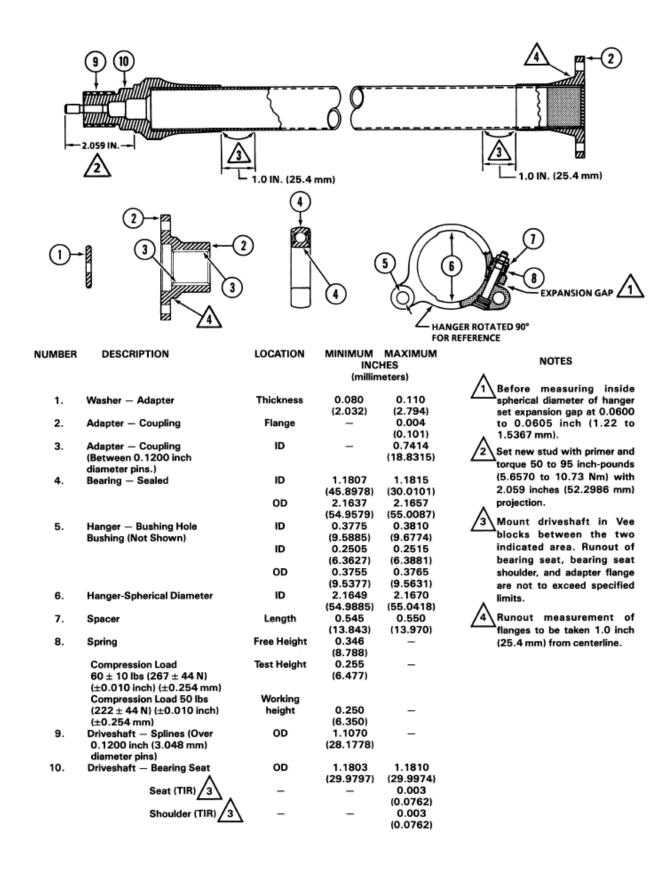
Figure 2 – Tail Rotor Segmented Driveshaft Assembly Wear Limits
