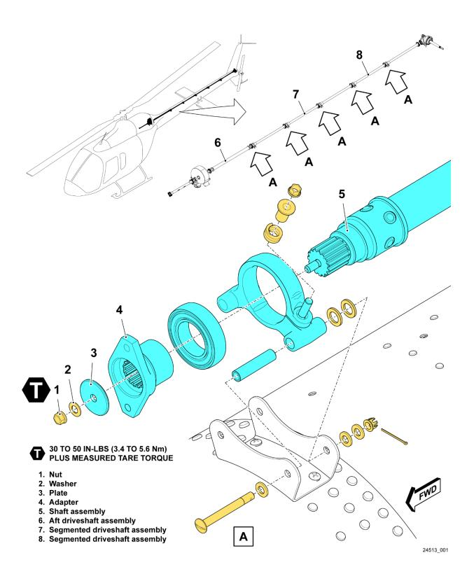
Figure 1 – Tail Rotor Segmented Driveshaft Assembly
