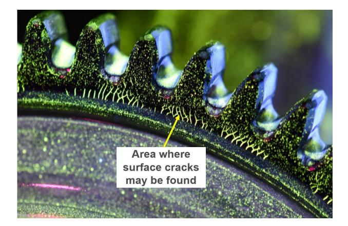
Figure 1. Area where surface cracks may be found.
