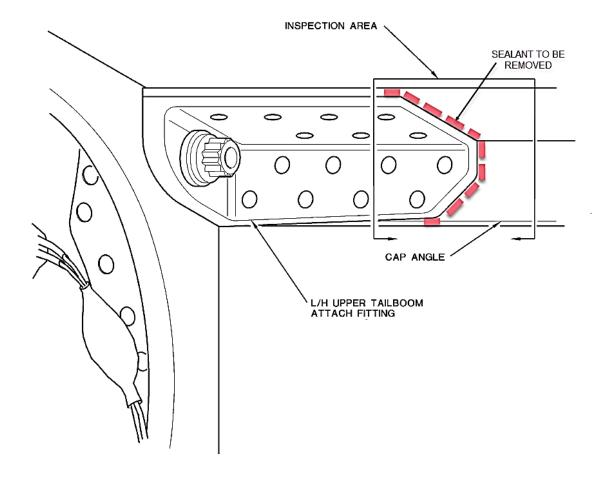
Figure 1. Fuselage Tailboom Attachment Inspection.
