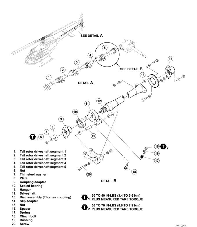
Figure 1 - Tail Rotor Drive System
