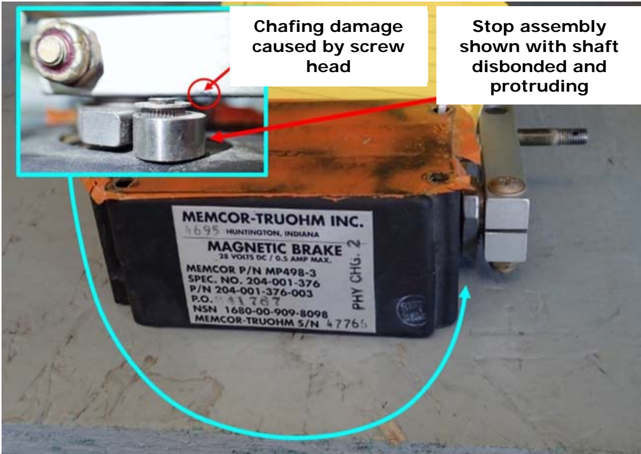
Figure 3. Stop assembly with disbonded shaft.
