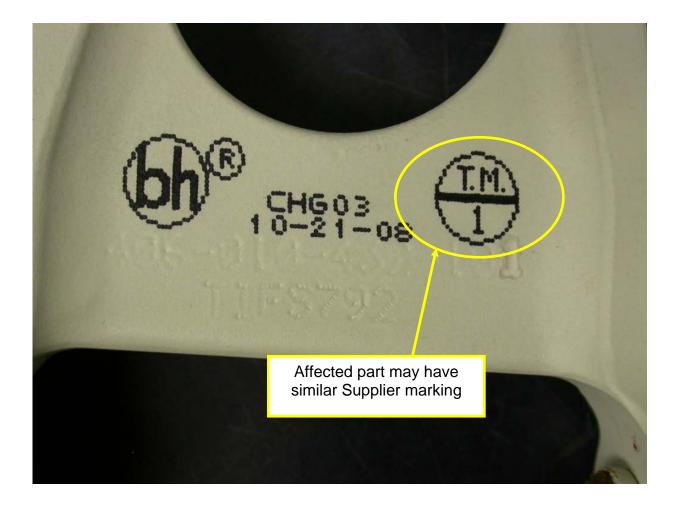
Figure 1. Affected part Supplier marking.
