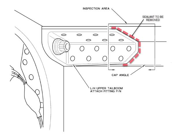
Figure 1. Fuselage Tailboom Attachment Fitting Sealant Removal.
