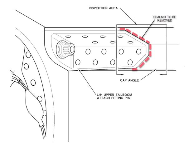
Figure 1. Fuselage Tailboom Attachment Inspection.
